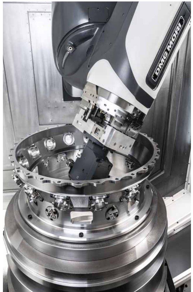
DMG MORI angle-head turbine housing
